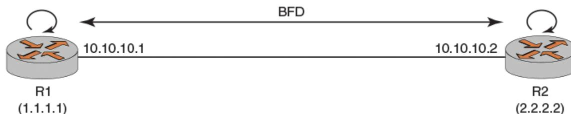
BFD works with both peers that are connected directly and peers that are multiple hops away. No automatic discovery of BFD neighbors occurs; the sessions must be explicitly configured for each new system. For more information about BFD, refer to RFC 5880, *Bidirectional Forwarding Detection (BFD)*, at <https://tools.ietf.org/html/rfc5880>.
