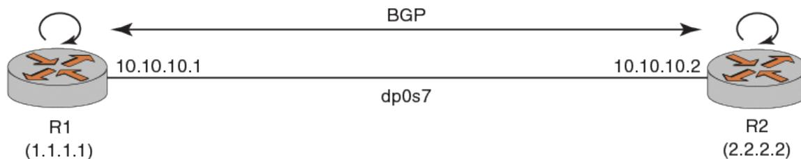
To configure BFD for BGP single hop by using IPv4 addressing, perform the following steps in configuration mode.
